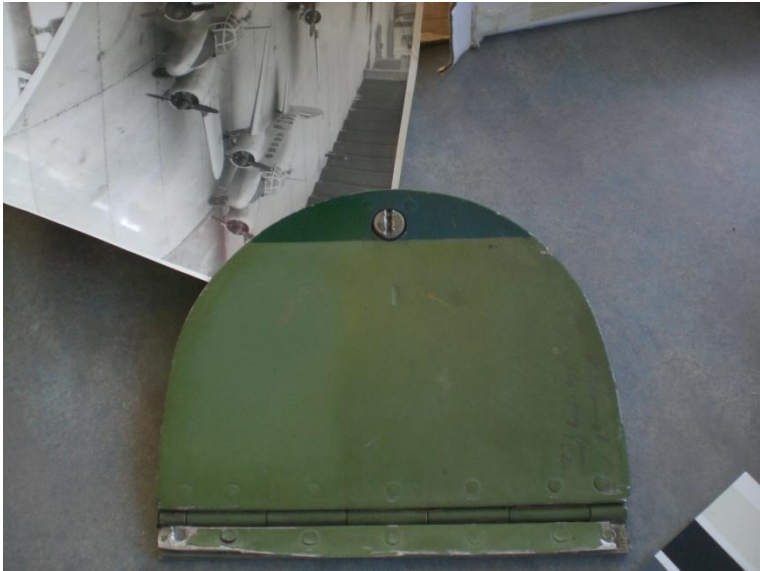
Sample 1: left hand side has been cleaned with de-ionised water using cotton buds.
